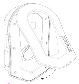
Step 2: Add fascia to the enclosure cover of the zappi as shown.
