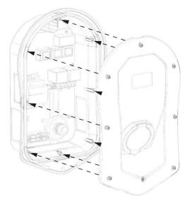
Step 1: Offer cover to the enclosure, ensuring all cables are neatly secured inside the unit.
