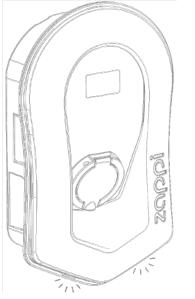
Step 3: Ensure the 2 tabs at the bottom of the Step 4: zappi is now ready for operation. fascia click to indicate its securely fixed in place.
