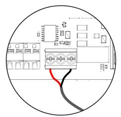
If the eSense input is provided using an external volt-free contact then this must be connected to the outer terminals marked "24V out" and "in"
