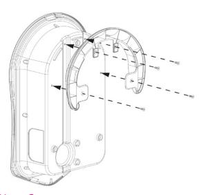
**Step 2:** If installing a tethered zoppi, you must ensure the cable wall guard is fixed to the unit using the 4 screws supplied.
