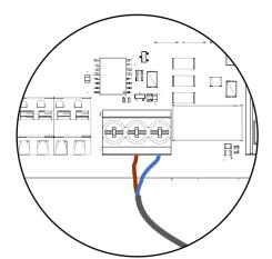
If the eSense signal is provided by using an external voltage this must be connected to the two right hand terminals marked "24-230V AC/DC in"
