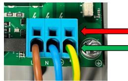
Release Lever (DO NOT INSERT CABLES!)
