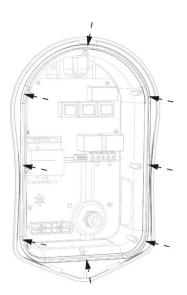
Step 7: Secure the unit to the wall using the fixing Step 8: Ensure O-ring is present and sits neatly kit provided. Ensure the grommets are used to into its channel. maintain its IP integrity.
