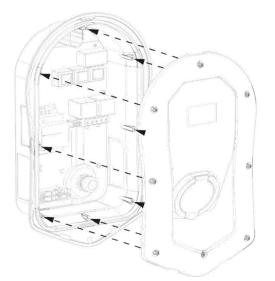
Step 1: Offer cover to the enclosure, ensuring all cables are neatly secured inside the unit.
