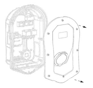
Step 3: Remove all 8 screws from the enclosure and carefully lift away.
