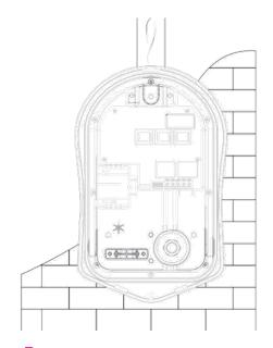
**Step 5:** Using zappi template mark mounting holes. For fixing to brick, use the top and 2 bottom holes (left/right). Use the 2 vertical holes as well as the top hole if mounting to a stud wall or joist.
