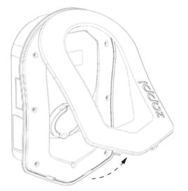
**Step 1:** Carefully remove fascia from the zoppi by pressing the 2 clips located at the bottom of unit inwards whilst pulling the fascia towards you.
