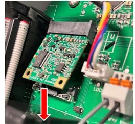
**Step 8:** Before closing the zappi check that none of the surrounding cables or connections have been loosened or disconnected.
