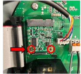
**Step 6:** Pull the board downwards and out of the socket on the top edge.
