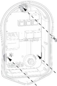
**Using the fixing kit provided secure unit to the wall ensuring the sealing washers are used to maintain its IP integrity.**
