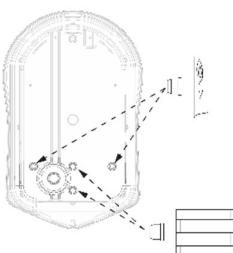
**To maintain the IP rating of the unit you must ensure that the bungs provided are inserted in any mounting holes that are not used.**
