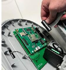
Unscrew the cover and unclip flat ribbon cable.
