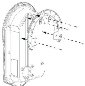
If installing a tethered zappi you will need to fit the enclosed cable wall guard to the unit using the **4x 4mm x12mm** screws supplied.
