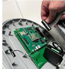
Re-fit the cover ensuring the ribbon cable is seated firmly, both in the zappi and onto the back of the cover.
