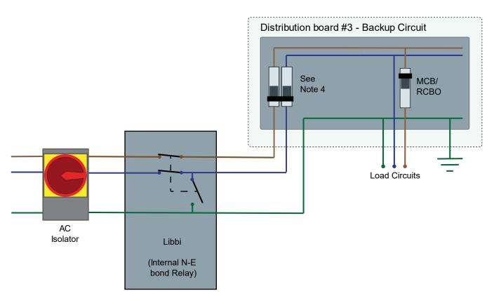
N-E Circuit for On-Grid Conditions
