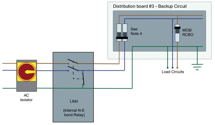
N-E Circuit for Off-Grid Conditions
